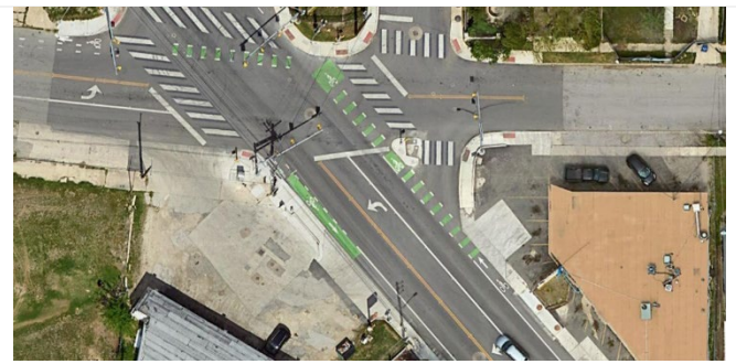
Right slip-lane allows cars to cut across the bike lane. Example at the intersection of Fredericksburg Road and Cincinnati Avenue.
