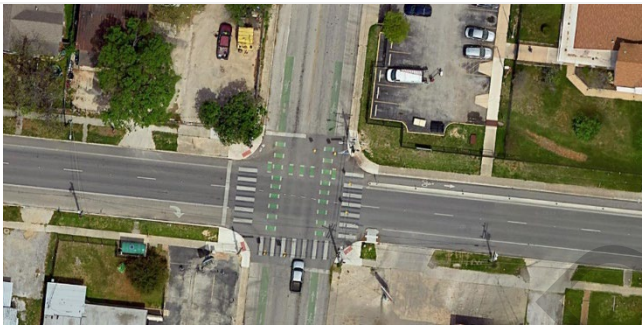
High-visibility green conflict markings at the intersection of Buena Vista Street and Trinity Street help increase the visibility of people biking.
