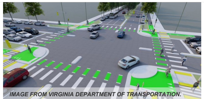
Protected intersections are designed to maintain separation for people biking from vehicle traffic as they travel through the intersection.
