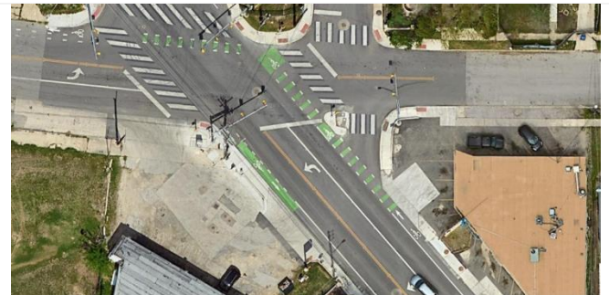
Right slip-lane allows cars to cut across the bike lane. Example at the intersection of Fredericksburg Road and Cincinnati Avenue.
